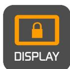
The Display off function allows for the screen to be turned off with out effecting the operation of the unit. This is combined with the screen lock function and will become active by tapping the power on/off button on the side of the unit.
