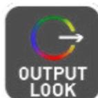
**OUTPUT LOOK** – With this option the selected LOOK is also applied to both the SDI and HDMI loop outs of the Sumo 19. This will allow for review on a larger monitor or to be used with a wireless sender. This function can also be combined with the down convert option that can be found in the input menu.
