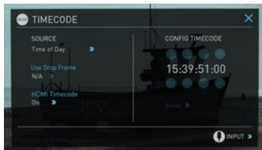
With this setting, each new clip that is created will contain embedded Timecode starting with the time of day when the recording is started. Please check that Sumo19 clock has been set correctly.
