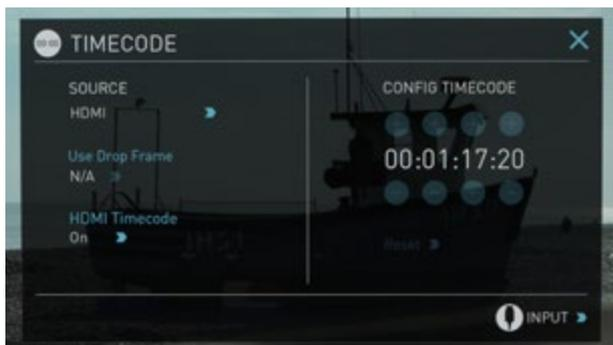
With this setting, the SDI or HDMI input will use the Timecode embedded in the input signal. The controls to adjust the Timecode value are disabled in this menu as you will need to adjust these on the camera. Note that not all HDMI sources embed Timecode.
