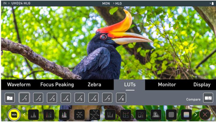
Atomos support 3D LUTs in the industry standard .cube format and provides up to 8 LUT memory slots for you to load your LUTs in to.
